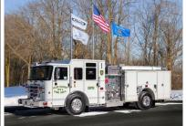
(New) Engine 1372: 2016 Pierce Enforcer, 8 man fully enclosed cab, 1500 gallon per minute Two-Stage Pump, 500 gallon tank, 10Kw Harrison hydraulic generator, Whelen light package, enclosed ladders/tool storage, Bullard infrared camera, Motorola APX6500 mobile & Tait TP8115 portable radios.
