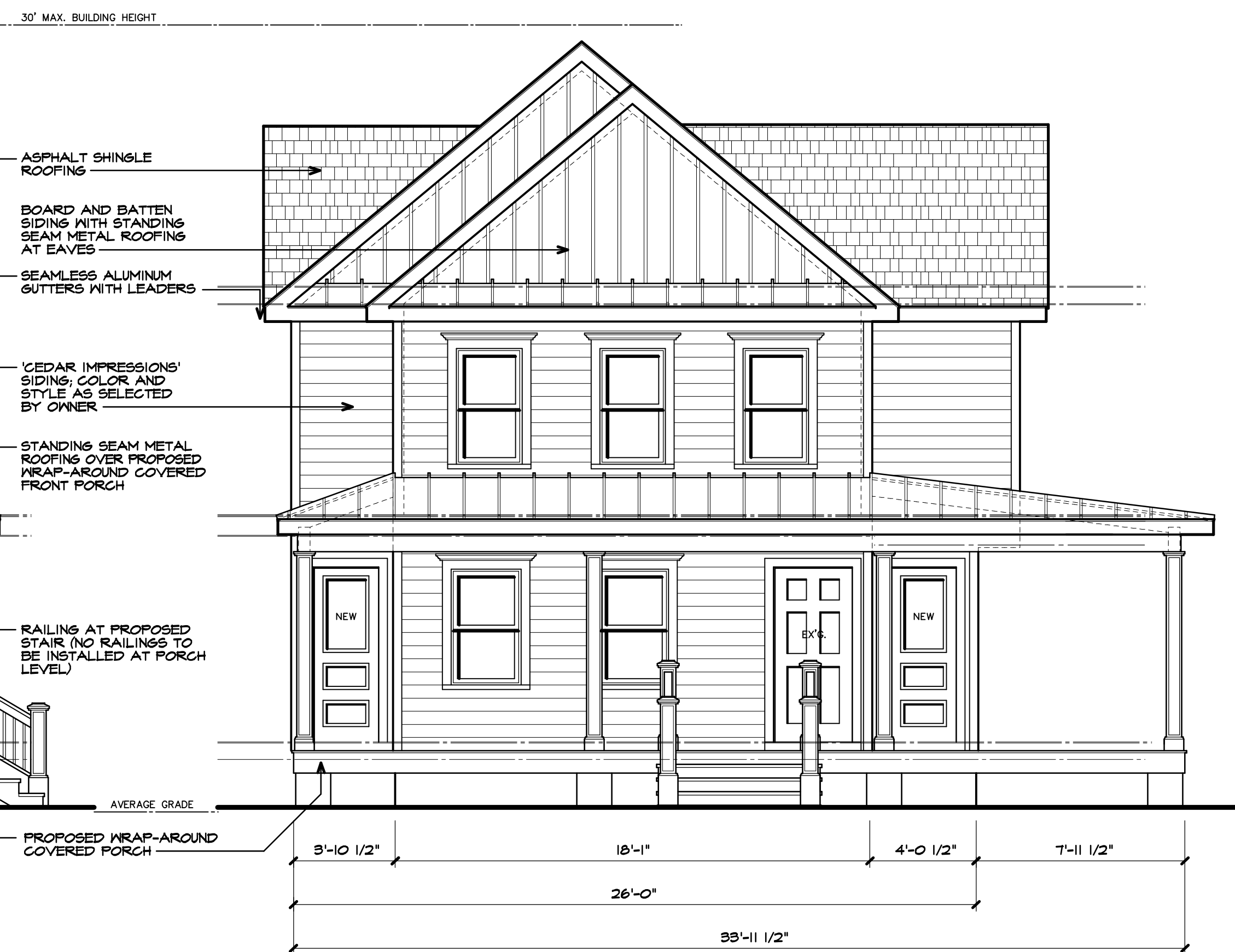
PROPOSED FRONT ELEVATION (WILLOW STREET) SCALE: 1/4" = 1'-0"
