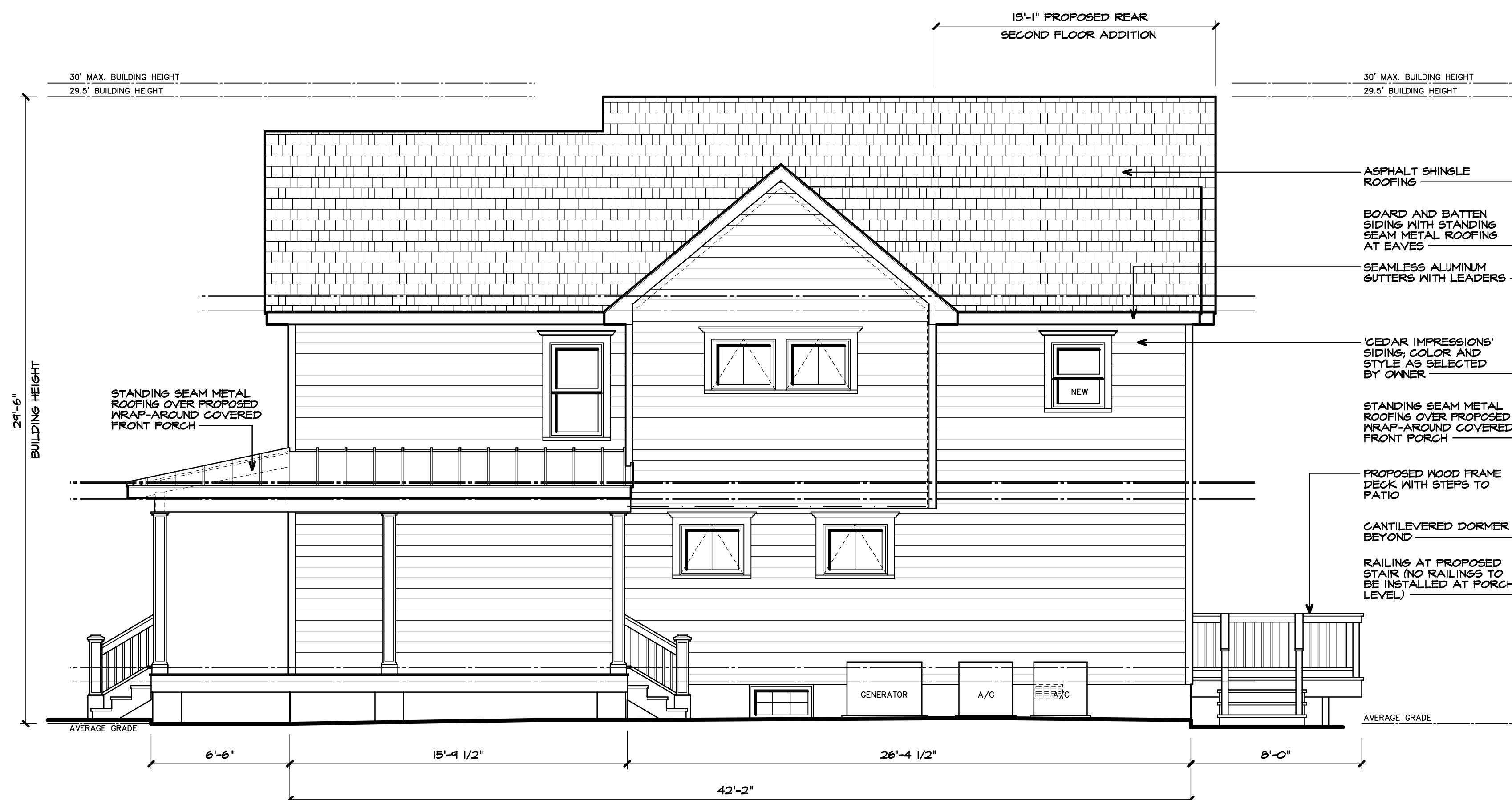
PROPOSED RIGHT SIDE ELEVATION SCALE: 1/4" = 1'-0"
