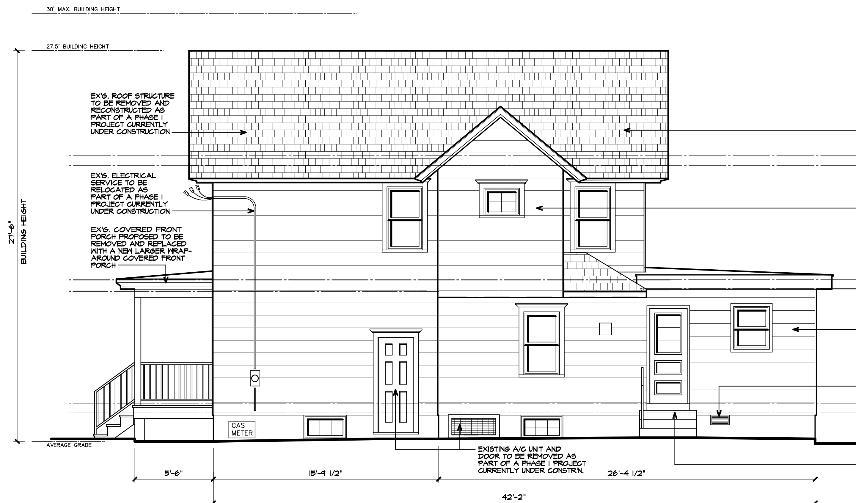
EXISTING RIGHT SIDE ELEVATION SCALE: 1/4" = 1'-0"
