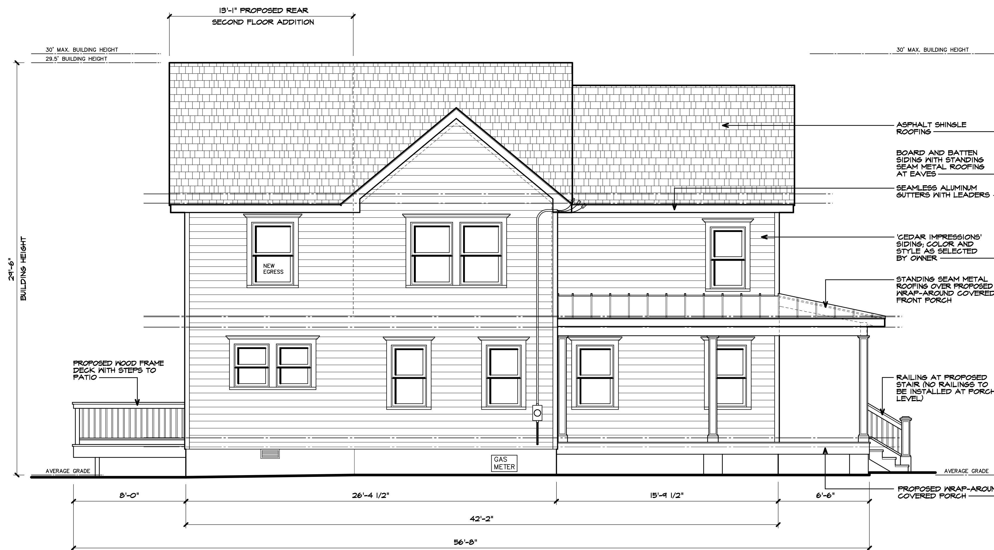
PROPOSED FRONT ELEVATION (OAK PLACE) SCALE: 1/4" = 1'-0"
