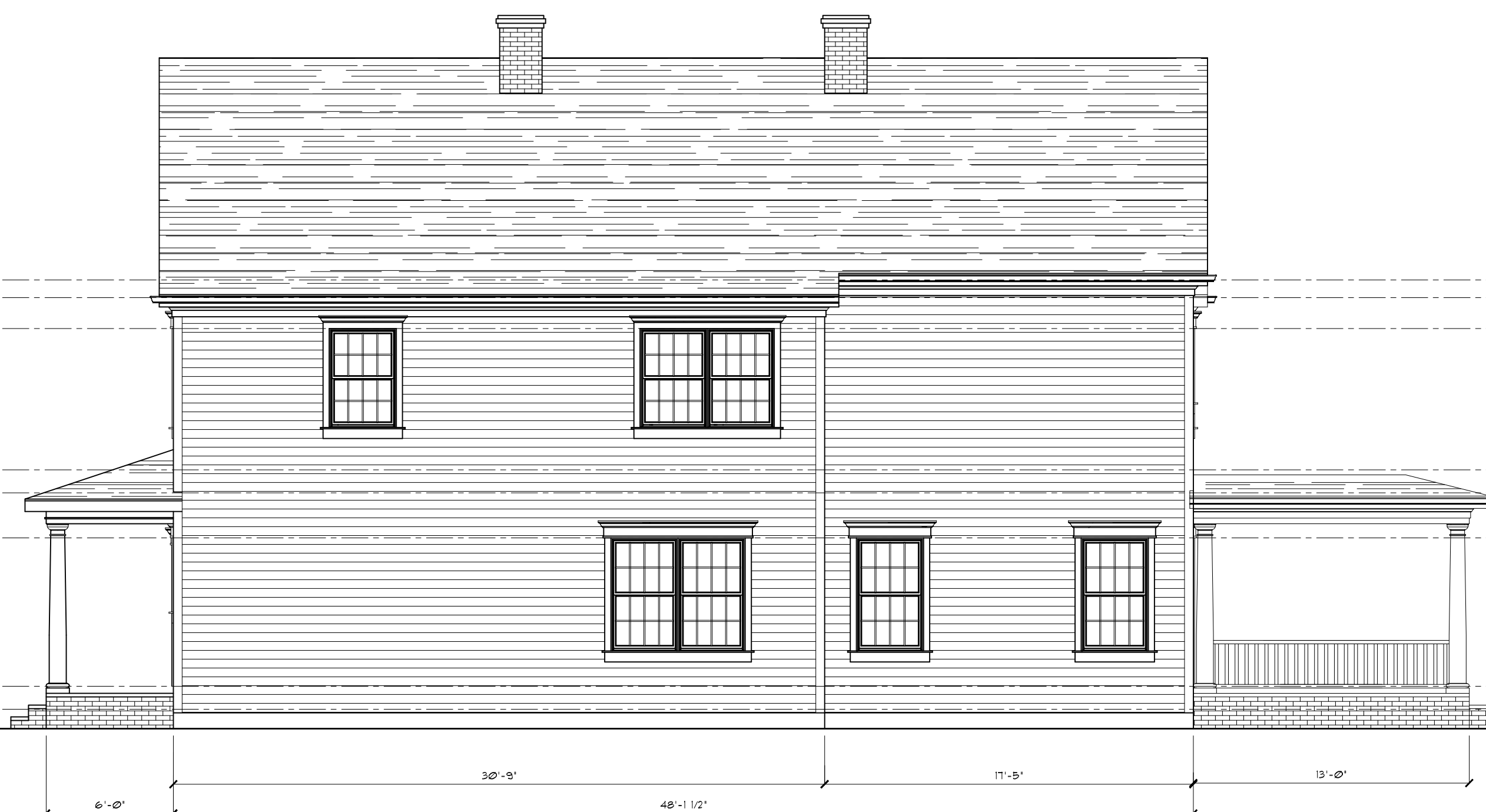
REAR ELEVATION SCALE: 3/16" = 1'-0"
